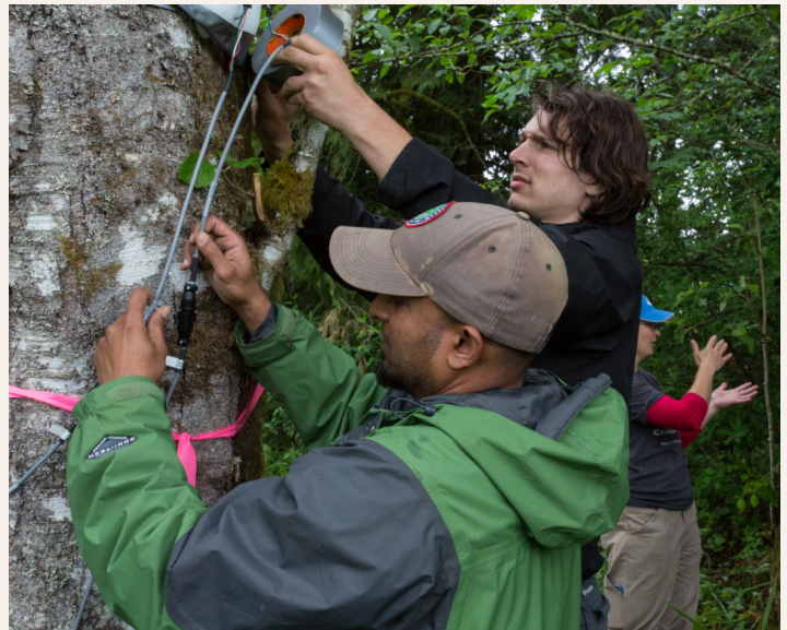
Above, Ani Jayakaran, installing sap flux sensors to measure tree water use.
